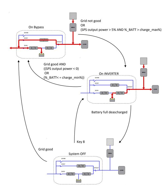
SPS output power (express end in %) is positive if exit from SPS and supply the load charge\_min\_% and charge\_max\_% are the value set in the menu. Standard value are respectively 30% and 50%
