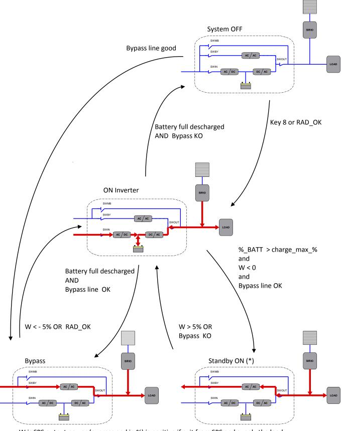
W is SPS output power (express end in %) is positive if exit from SPS and supply the load charge\_max% is the value set in the menu. Standard value is 95% When %\_BATT > charge\_max\_% rectifier is disabled.
