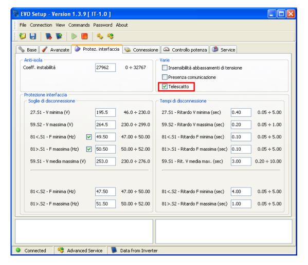
With the selected parameter checked, solar inverter stops when SPS switch to bypass line. It is request when non energy can be injected into the grid.
