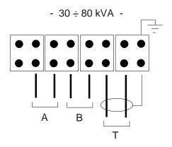
A = connection to external output SPS switch auxiliary;
